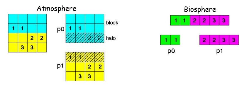
Flexible communication scheme (remapping, sub-objects, time shifts) for atmosphere biosphere coupling
