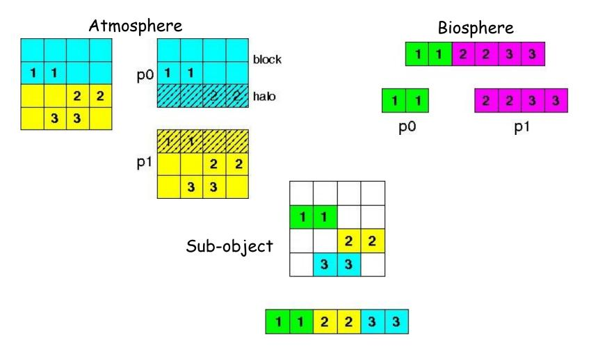
Flexible communication scheme (remapping, sub-objects, time shifts) for atmosphere biosphere coupling
