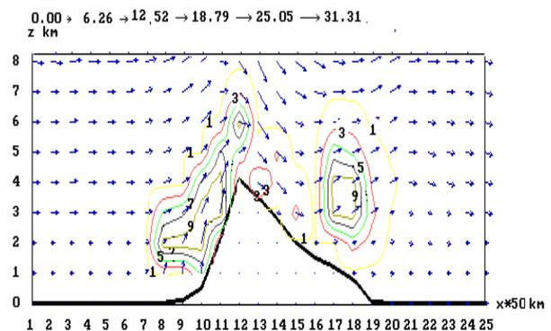
**Figure 4.** Distribution of the wind velocity (m/s) and the atmospheric water ( $10^{-1}\text{g/kg}$ ) in the latitudinal section  $X0Z$  ( $y = 13 \times 50\text{km}$ ) at the moment  $t=4\text{ p.m.}$
