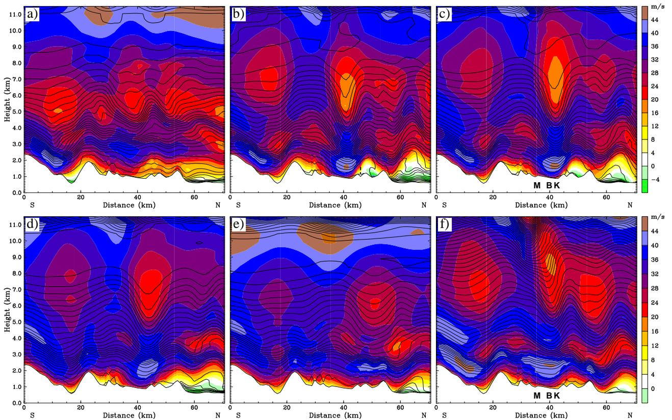
**Figure 4:** Vertical cross-sections of potential temperature (contour interval 1 K) and wind speed (see colour key) along line a1-a2 indicated in Fig. 1. Results are shown for the reference experiment at (a) 03 UTC, (b) 06 UTC, (c) 07 UTC, (d) 08 UTC and (e) 10 UTC, and for the sensitivity test with modified stratification at 07 UTC (f). In (c) and (f), the locations of Mittenwald (M), Buckelwiesen (B) and Krün (K) are indicated.
