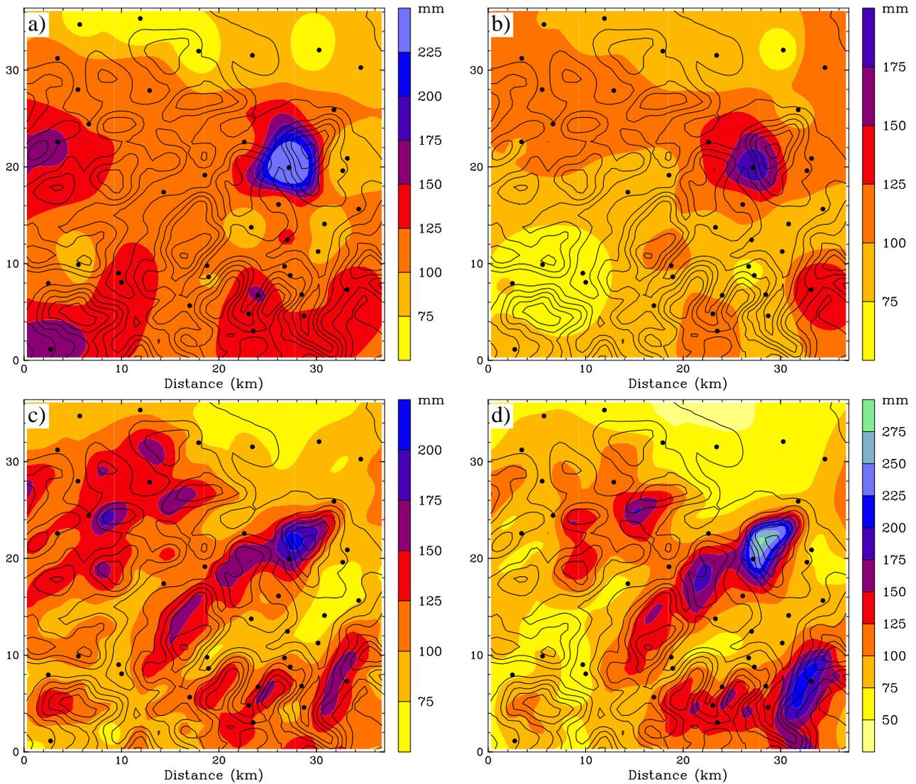
**Figure 3:** Accumulated precipitation fields in the analysis domain for 0600 UTC 10 July – 0600 UTC 12 July 2005 (left column) and 1800 UTC 15 August – 0600 UTC 17 August 2005 (right column). Model topography is contoured every 400 m, and black dots indicate rain gauge stations. The upper (lower) panels show interpolated observed (simulated) precipitation.
