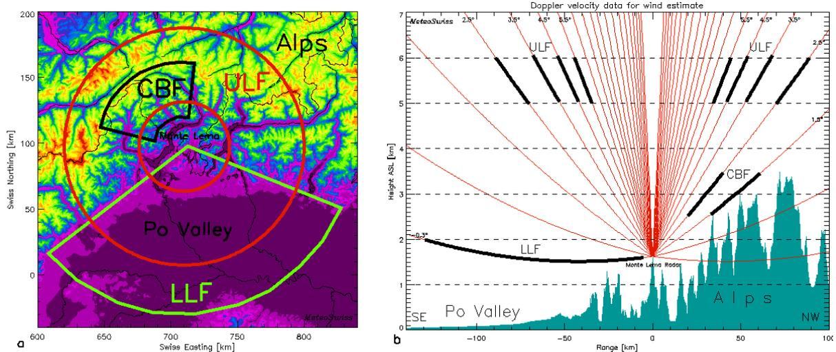
**Figure 1:** (a) Location of the three areas in which LLF, CBF and ULF are estimated; Monte Lema radar is at the centre of the picture. (b) Vertical cross section showing the 20 elevation angles of Monte Lema radar scan strategy (red lines) and the regions selected for the estimate of the three flows (thick lines).
