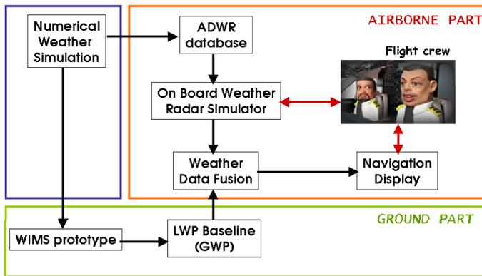
**Figure 1:** Weather simulation products integration in the Flight Simulator
