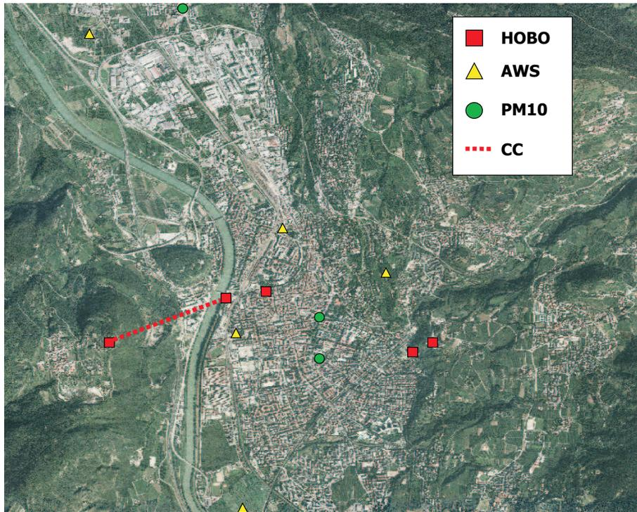
**Figure 1:** Schematic representation of the layout of the instrument network, including HoBo air temperature and humidity sensors (red squares), automated weather stations (AWS, yellow triangles), air-quality stations (green circles) and a measurement system based on a cable car (dotted red line).
