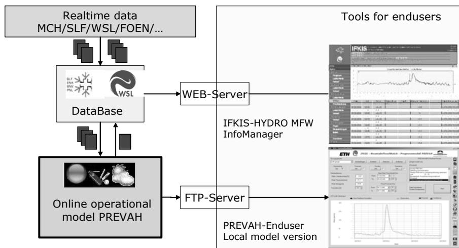
Figure 3: Work flow of the forecast model PREVAH, as implemented in Canton Glarus for real time runoff nowcasting and forecasting. Screen shots of the IFKIS-Hydro web platform.
