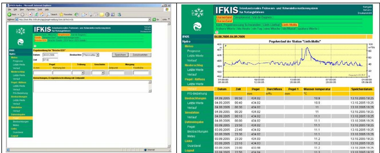
**Figure 2:** Screen shots of the IFKIS-Hydro web platform. The left image shows the screen where observations at a site as shown in figure 1 can be entered. The right image shows a measured hydrograph
