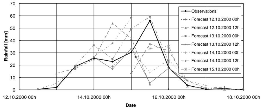
**Figure 2:** Mean predicted rainfall volumes over 12 hours periods on the Upper Rhone River catchment area for 7 different forecasts, comparison with mean observed volumes.
