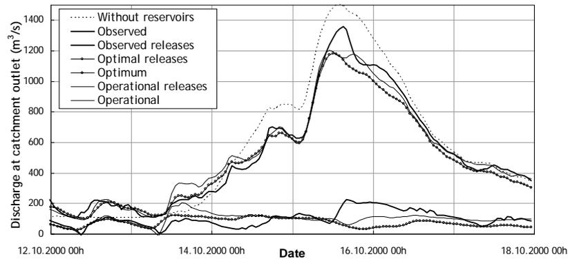
**Figure 4:** Flood hydrographs during the October 2000 event. The hydrographs without reservoirs, without preventive turbine operations and with optimized turbine operations are compared.
