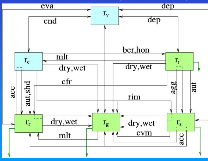
eva=evaporation dep=vapor deposition cnd=condensation hen=heterogeneous nucleation ber=Bergeron-Findeisen hon=homogeneous nucleation mlt=melting dry, wet=dry and wet growth acc=accretion aut=atoconversion shd=water shedding cfr=contact freezing agg=aggregation rim=riming cvm=conversion melting
