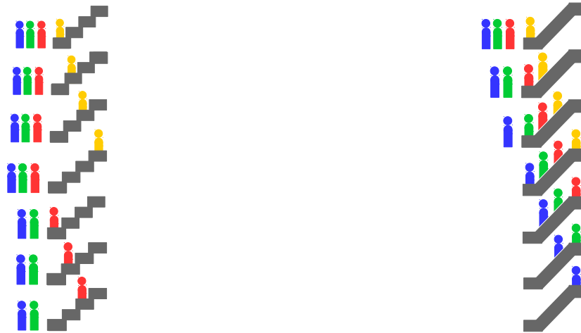
Figure 2.1: Analogy : vector pipelining like mechanic stairs (right) against an elevator for a scalar unit (left)
