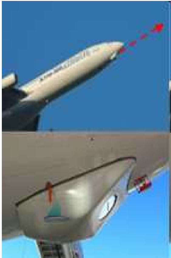
Forward looking turbulence/gust UV LIDAR beneath A340-300 cockpit
