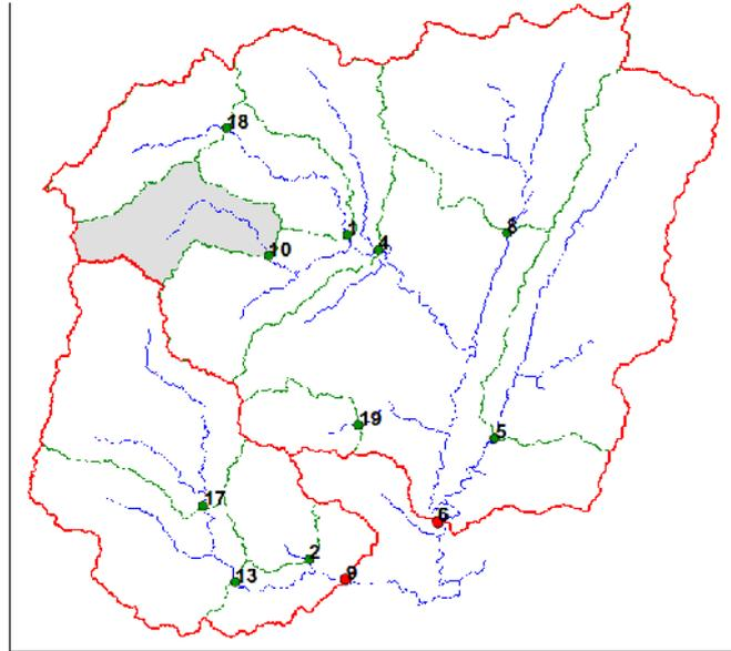
Fig. 2. Map of the two main sub-basins proposed for calibration (red) and the remaining 10 sub-basins (green). The numbers refer to basin identification as in table 2. The major river network is figured in blue, as well as the limits of the ALMIP domain (black rectangle). The greyed area is the Dong basin selected for the sub-meso scale experiment (see next section).
