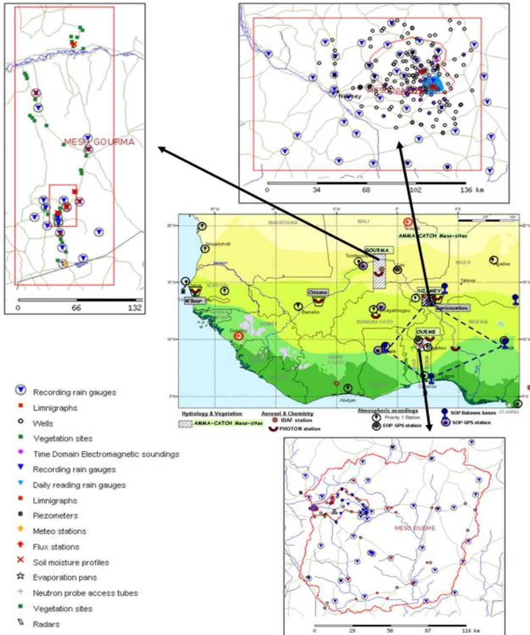
Fig. 1: The three mesoscale domains are shown with the locations of observation sites indicated using symbols defined in the figure at the lower left. The AMMA-CATCH region consists in a north-south transect encompassing the three meso-sites. Finally, the Ouémé catchment is shown in the lower right, with the Donga sub-basin in the northwestern part of the domain.
