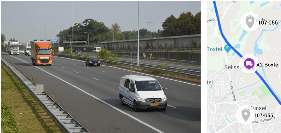
Figure 1: Left: The truck in which fuel consumption was measured was preceded at about 50 m by a van with a pole measuring wind parameters. The picture is taken at a stretch of the route with solid sound barriers. Right: location of Harmonie-Arome grid-points (grey balloons) near the A2 highway (blue line) near Boxtel.
