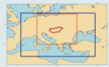
The two clustering domains of the ECMWF/ALADIN ensemble system. (The larger clustering area is the same as the integration domain of the ALADIN model)
