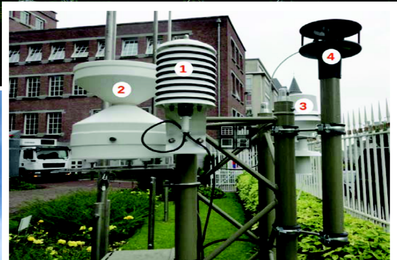
Figure 4. Detailed view of the sensors at one of the weather stations: actively ventilated radiation shield (1) with temperature sensor, rain gauge (2), passively ventilated shield (3) with temperature and relative humidity measurement, and sonic anemometer (4).
