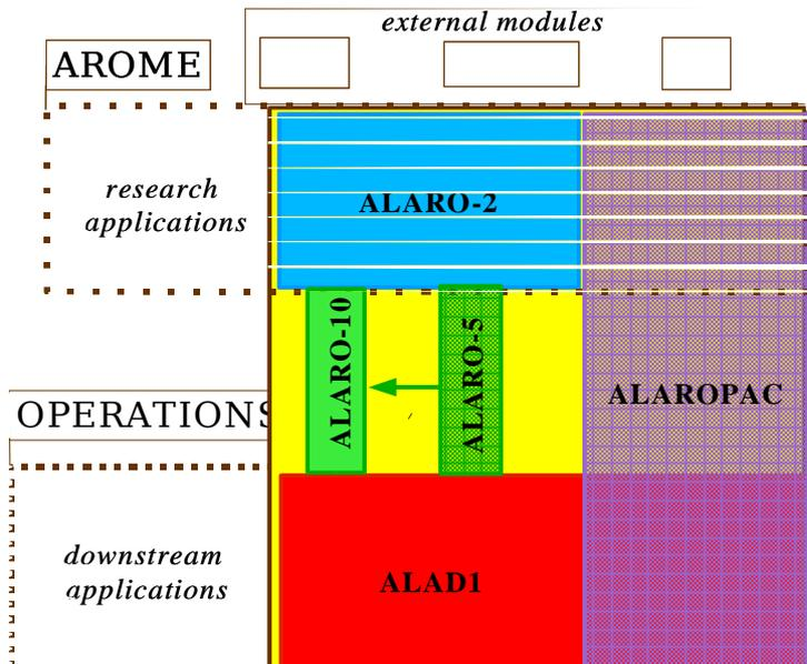
The "toolbox" concept aims at being able to run operational NWP suites on a broad range of scales and with different assimilation methods, using a "single" source code (*IFS/ARPEGE/ALARO*). Strategy for physical parameterizations may be based on downscaling (e.g. from ARPEGE/Climat to ARPEGE/NWP), upscaling (ALARO-10) or both (ALARO-5).
