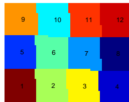
Checkerboard partitioner for LAM grid
