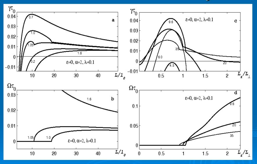
The growth rate of the convective-shear instability and frequencies of the generated convective-shear waves.
