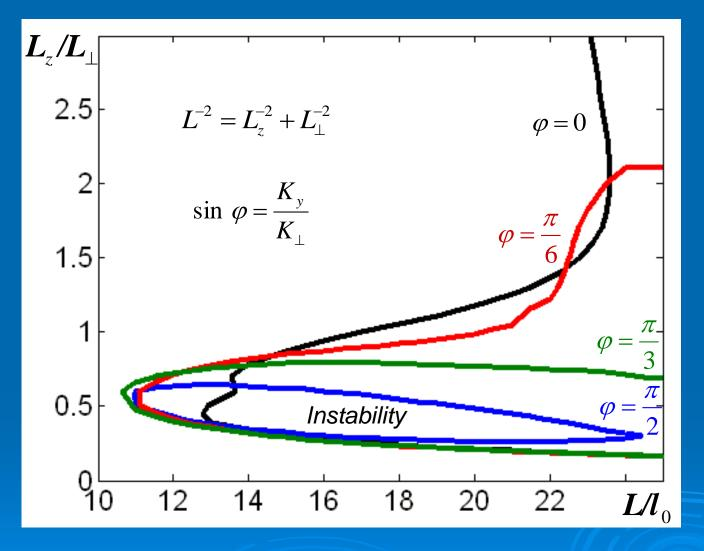
The range of parameters  $L_z/L_\perp$  and  $L/l_0$  for which the convective shear instability occurs
