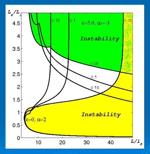
The range of parameters for which the convective-shear instability occurs for different values of shear and anisotropy.
