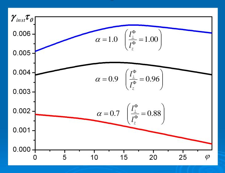
The growth rate of the convective shear instability for different thermal anisotropy
