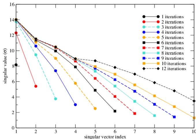
**Figure 3:** Singular values as a function of the number of iterations performed. It can be said that in general one needs about three times more iterations than the number of stable SVs desired. Experiments were performed on the supercomputer of Météo-France (which was a Fujitsu VPP5000 machine - "tora" - at the time of the experiments) with cycle30.
