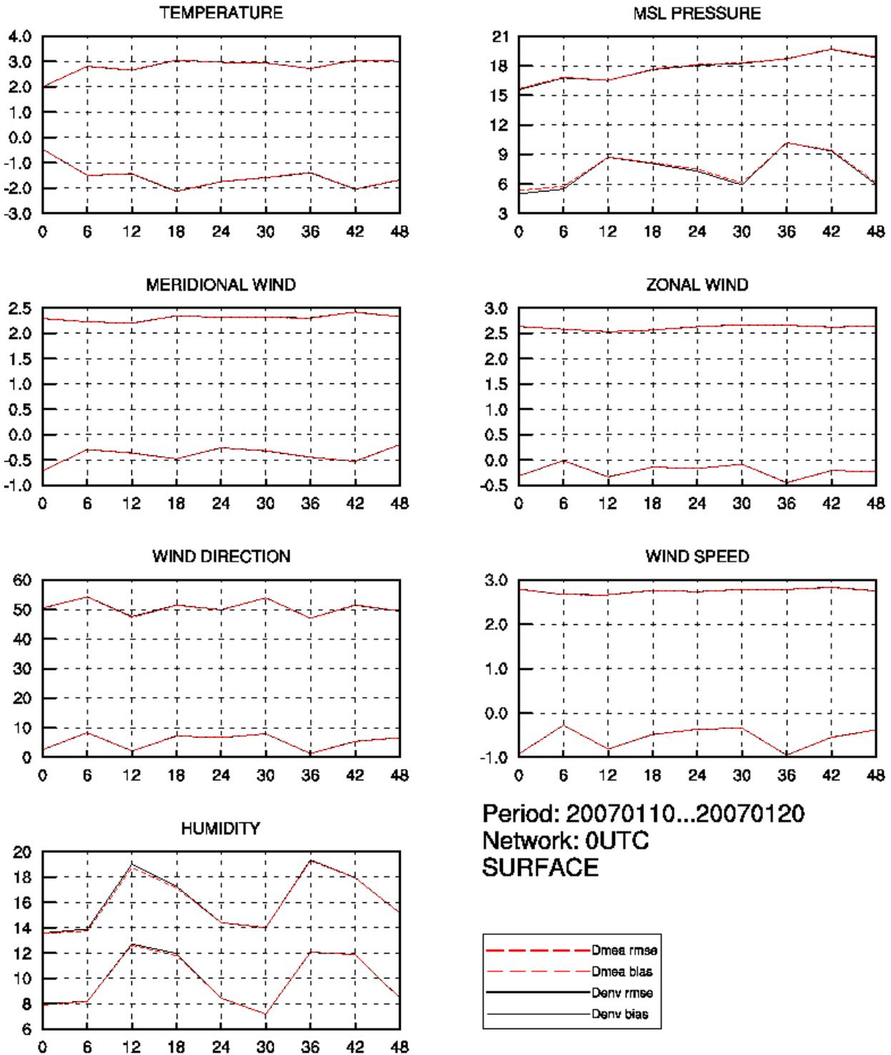
FIG. 2. Averaged skill scores of 10 model integrations driven by TCFs with mean and envelope orographies.
