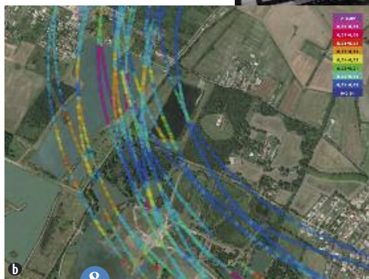
(a) Detection of GPS satellites. (b) GPS signal reflected by the continental surfaces.
