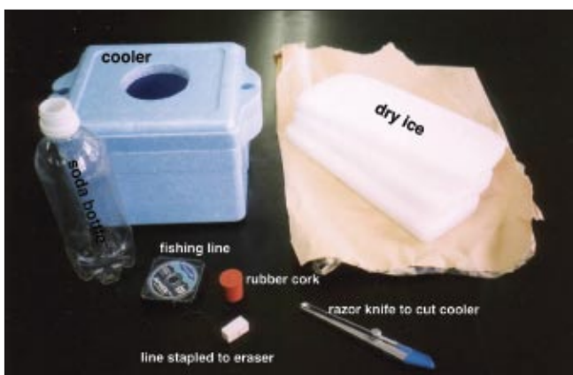
Fig. 1(b). Equipment needed to make and operate the snow crystal growth chamber.
