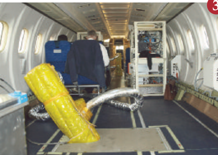
▲ CAROLS' installation in the ATR cabin (the antenna has a temperature regulation provided by the yellow cover)
