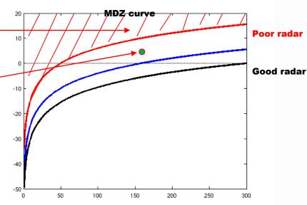
Minimum detectable Z as a function of distance from the radar
