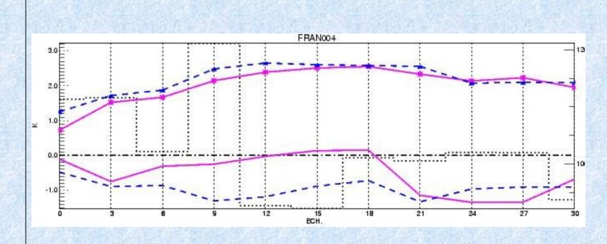
Fig. 5. Bias (bottom) and RMSE (top curves) of Arome (magenta) and Aladin (blue) forecasts in regards to SYNOP measurements for temperature. Abscissa is forecast range (hours).
