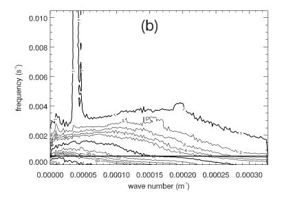
$\ln p_s$  decomposed between 0600 UTC and 1200 UTC of an anticyclonic case on 28 December 1999. The thick horizontal line corresponds to a filter cut-off period of 3 h.
