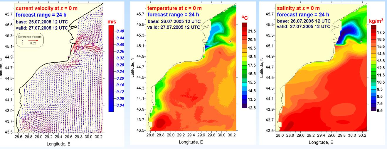
The current velocity (left), sea temperature (center) and salinity (right) 24h forecast of the POM circulation model for the Romanian coastal zone valid on 27.07.2005 12 UTC
