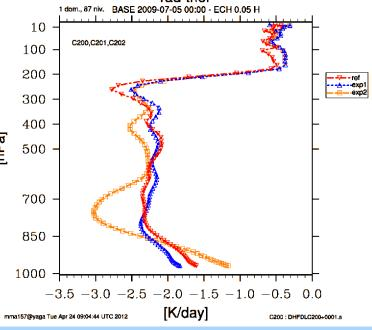
Figures show DDH cooling rates in thermal band for clear sky case. H2O without e-type continuum (left) and H2O with e-type continuum (right). RRTM reference in red, ACRANEB with old transmissions in blue and ACRANEB with new transmissions in yellow.
