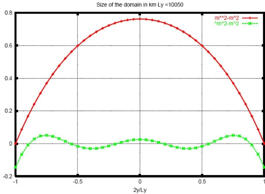
Approximation to the square **map factor real value** of the **Fourier estimation** with three coefficients ( $a_0$ ,  $a_1$  and  $a_2$ ) and of its **maximum value** in the domain.  $L_y = 10.050\text{km}$
