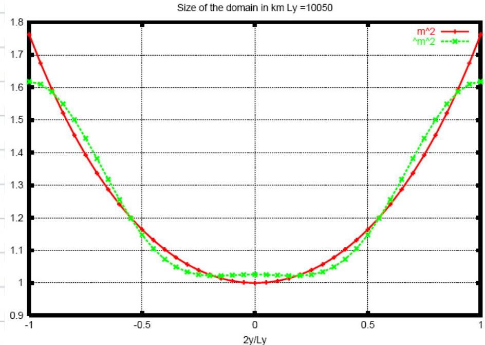
**Fourier estimation** of the square map factor with three coefficients ( $a_0$ ,  $a_1$  and  $a_2$ ) in comparison to the square **map factor real value**.  $L_y = 10.050\text{km}$
