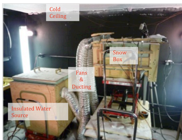
Figure 1: A) Experimental set up. The box on the lower left provides humidity-controlled airflow through a ducting system over the snow surface in the upper right. The temperature-controlled cold ceiling above provides the long wave radiation interaction.
