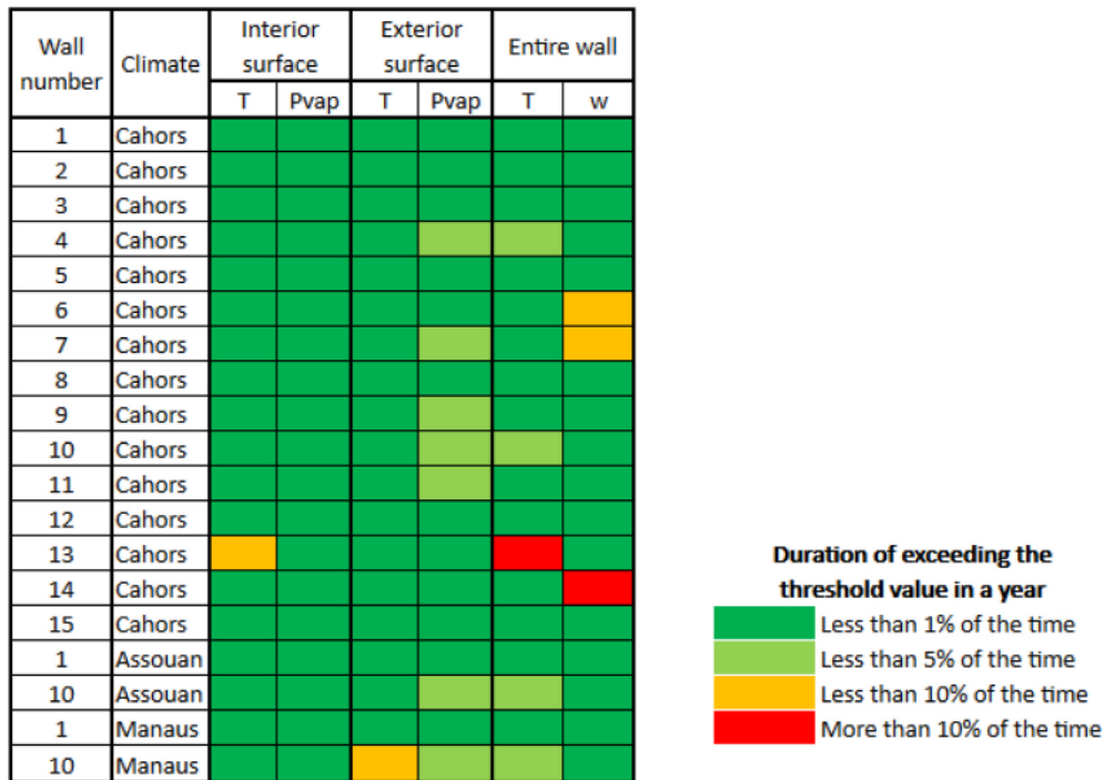
Fig. 8. Time during which the threshold value was exceeded in a year for each simulation with mesh version 2.
