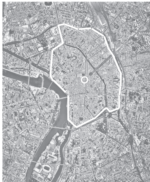
Fig. 2. Aerial photograph of the city centre of Toulouse: 3500 × 4400 m sample of IGN (Institut Géographique National) panchromatic image of June 24, 1998 (courtesy of IGN). The white continuous line approximately corresponds to an area of the old city centre that has been taken as the sampling area for extracting TIR directional anisotropy. The circle indicates the position of the central site.
