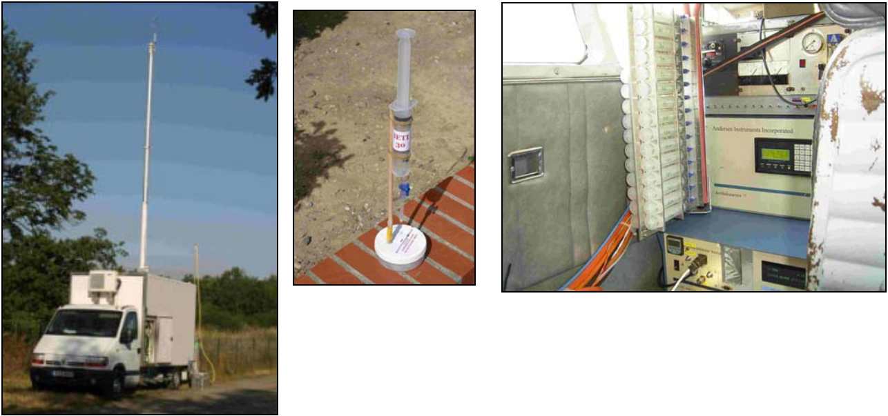
Figure 6: Instruments to measure SF_6 dispersion: a: The laboratory van equipped with a telescopic 10 m mast. SF_6 is released at 2m50 of height (seen behind the van). b: Ground sampling with a drop by drop system. c: Aircraft rack including 30 gas syringes.
