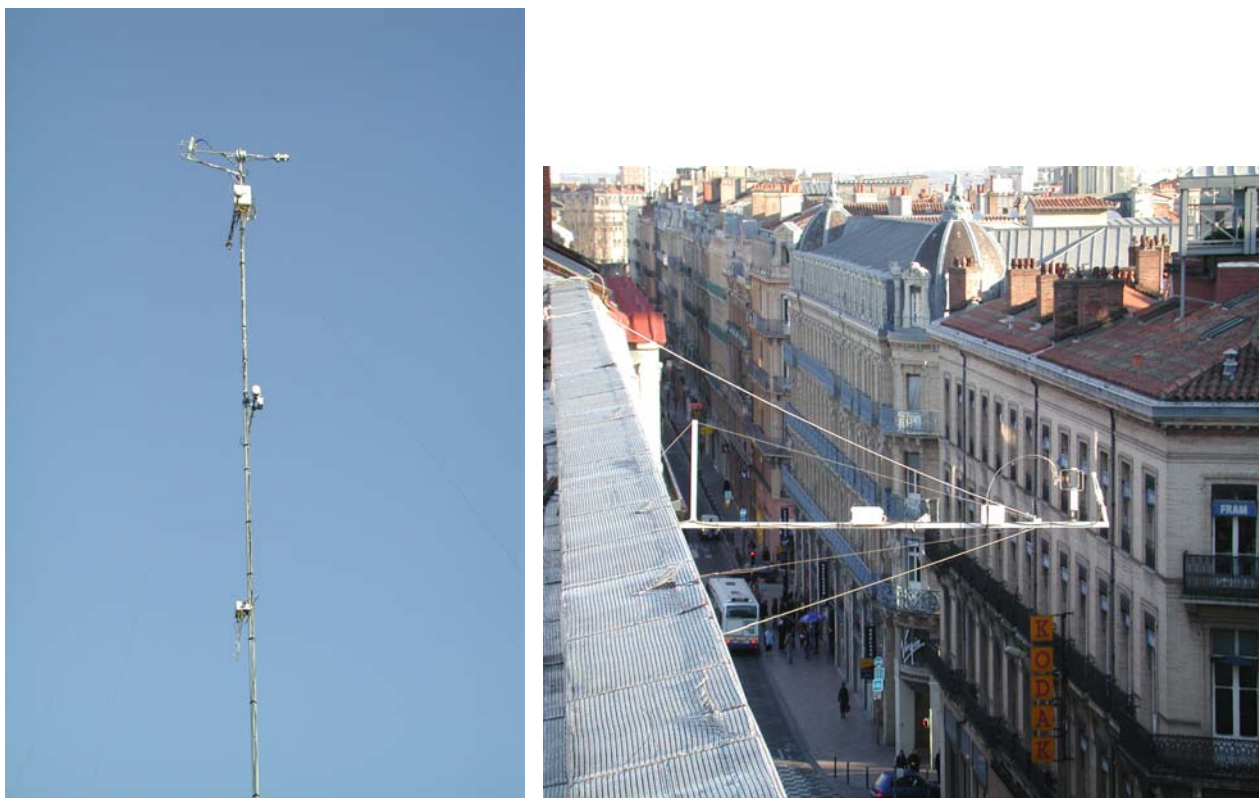
Figure 4: Left : the pneumatic tower for surface energy balance observations; Right: 5 m turbulence-aerosol measurement boom at the top of Alsace-Lorraine street canyon.
