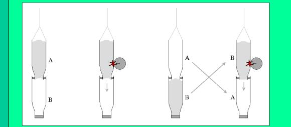
The granular phase transition is repeatable at will in both directions without significant change in density.
