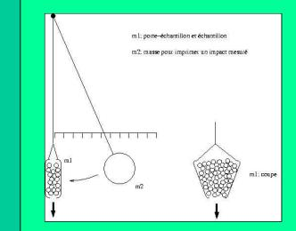
A rough estimate of GS cohesive energy can be derived from knocking energy. The energy barrier for the GS->GL transition is found between 0.01 J/dm<sup>3</sup> and 0.1 J/dm<sup>3.</sup> It obviously depends on grain size.
