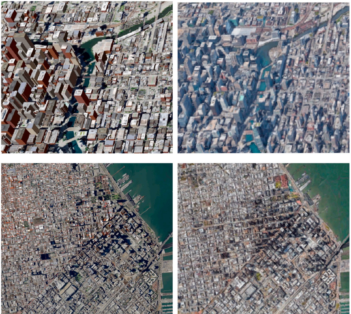
Fig. 8. Example DSC outputs. Left column: Views of cities using Google Earth. Right column: Similar views using automatically generated procedural model from DSC. Top row, Chicago, Bottom row, San Francisco.
