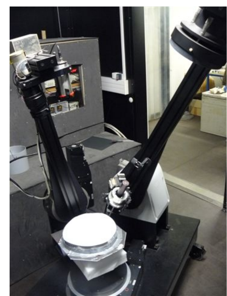
Figure 1 – S1 in the spectro-goniometer. Illumination in the right arm, the left arm is reflected light measurements.
